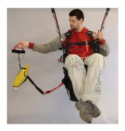
IMPORTANT: To prevent anomalous lateral loads, the bridle should be attached to both the loops on the shoulder straps. Not to just one of them.
